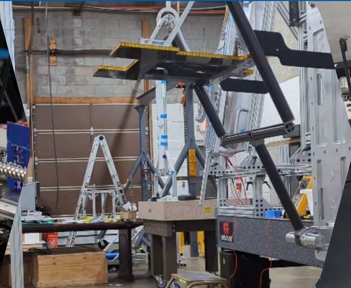
Completed IM-2 LTE/4G Rover Deployment Mechanism
