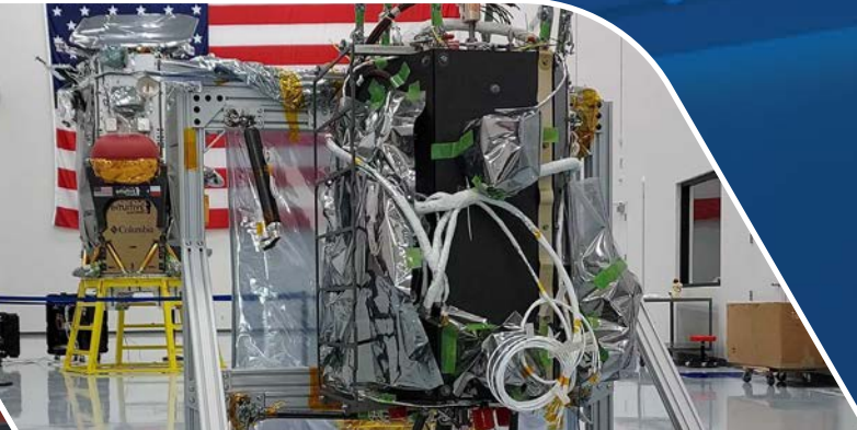
Micro Nova Hopper Undergoing Thermal Vacuum and Vibration Testing
