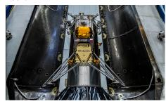
The Intuitive Machines Nova-C Nova-C class lunar lander completed all integration milestones and is safely encapsulated within SpaceX's payload fairing in preparation for launch.
