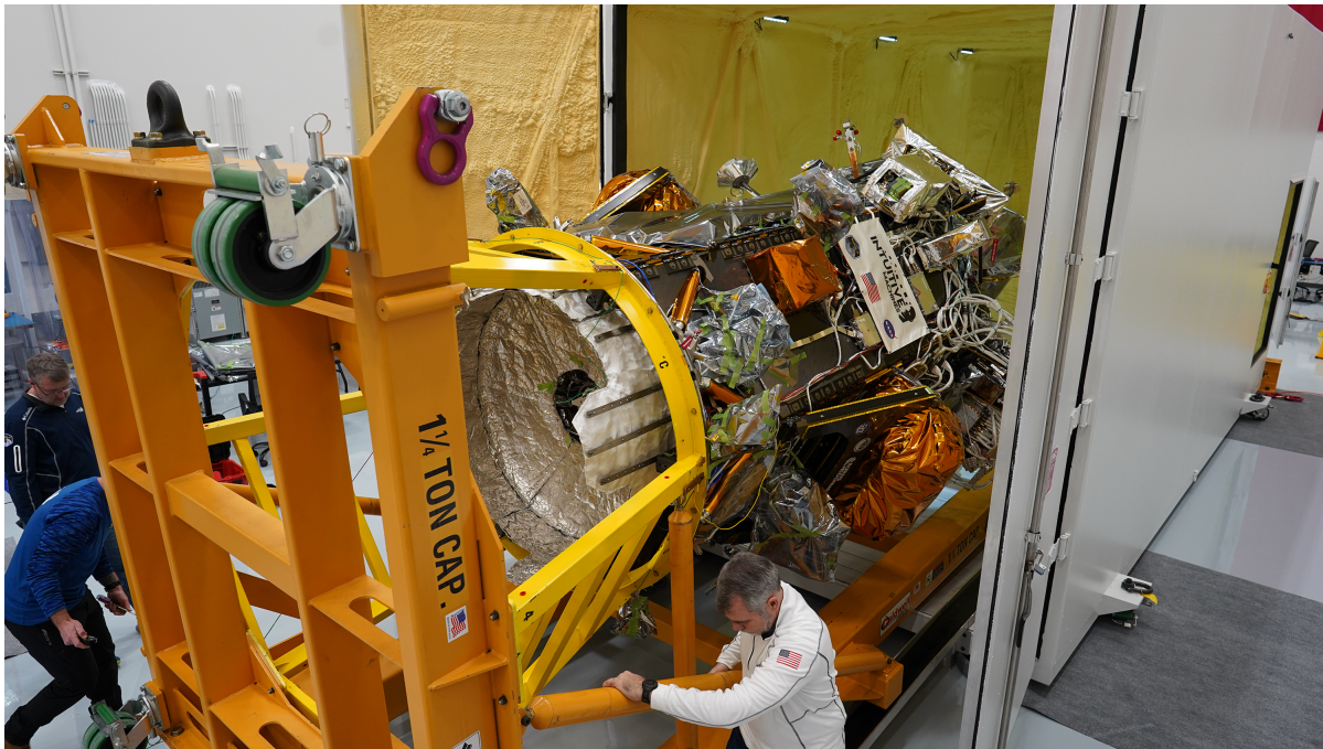
Figure 1: Intuitive Machines engineers loading the IM-1 mission Nova-C lunar lander into its custom container in Houston, TX.
