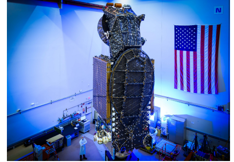
SXM-11, SiriusXM's newest satellite, is built on the IM 1300™ series platform.
