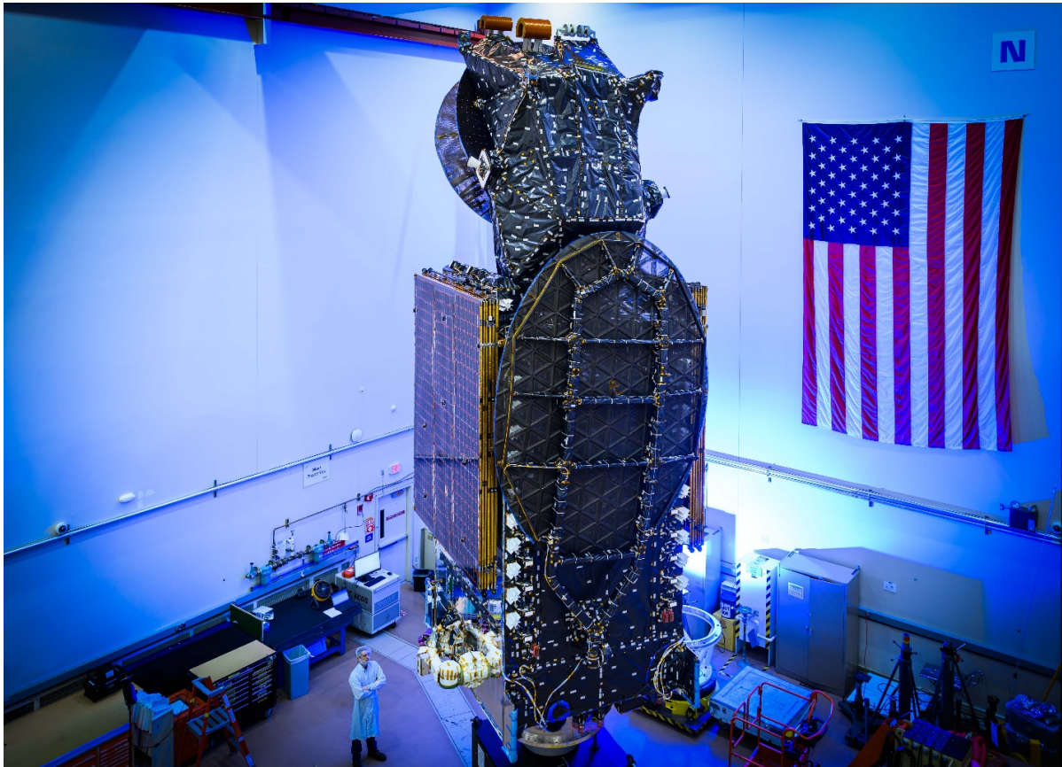
SXM-11, SiriusXM's newest satellite, is built on the IM 1300™ series platform.
